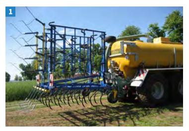
entire worked area. In addition, they are unsuitable for stubble fields, as they are prone to blocking. The new Treffler model presents a cultivator with a frame height of 70 cm. This height significantly reduces the risk of blockage. The pivot is positioned approx. 15 cm in front of the tine tip, which means that a tine encountering resistance is automatically pushed upwards, ensuring precision depth control (draft control). In spite of the
