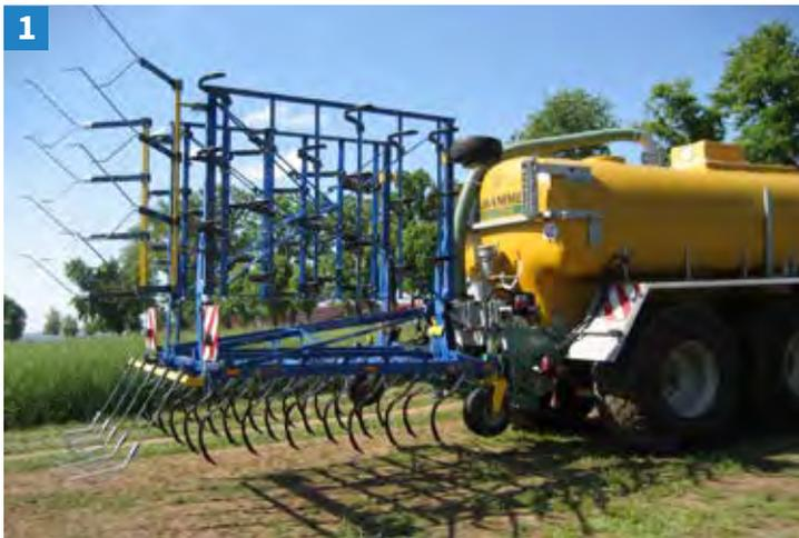
entire worked area. In addition, they are unsuitable for stubble fields, as they are prone to blocking. The new Treffler model presents a cultivator with a frame height of 70 cm. This height significantly reduces the risk of blockage. The pivot is positioned approx. 15 cm in front of the tine tip, which means that a tine encountering resistance is automatically pushed upwards, ensuring precision depth control (draft control). In spite of the
