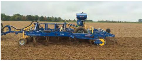
cm, the machine is the perfect tool to destroy cover crops. The roots of grass clover, lucerne and other grass covers as well as of dock leaves and other weeds are cut just below the surface, preventing second growth. The cultivator is designed to prevent blocking and can thus be used to work fields with high and bulky harvest residue such as rain-flattened cereal crops and forage corn stubble. Even running over the
