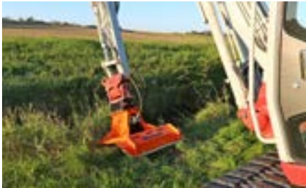
Optional: Cylinder swivel mechanism.
