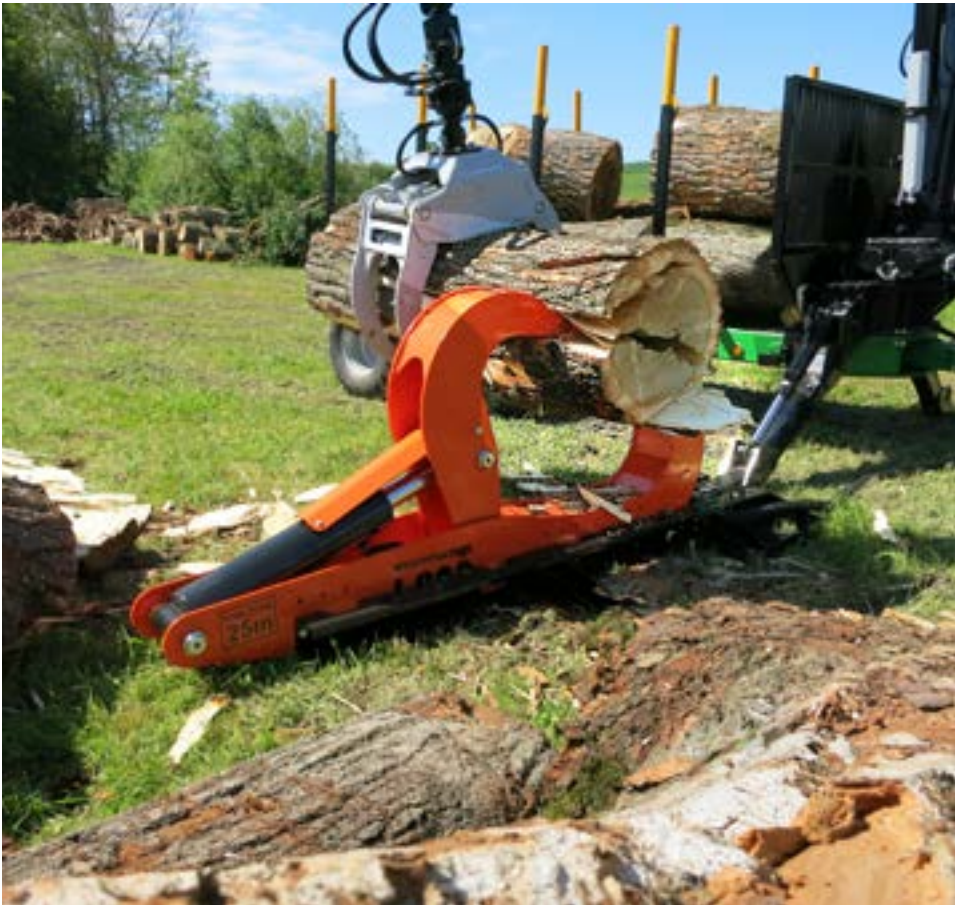
The trunk can be split and loaded in one work step.
