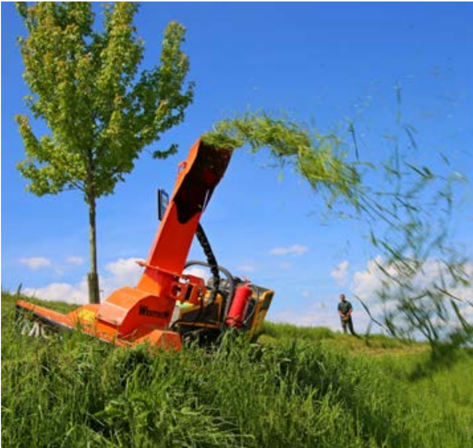
The Mowblower® can be mounted to a remote-controlled mower.
