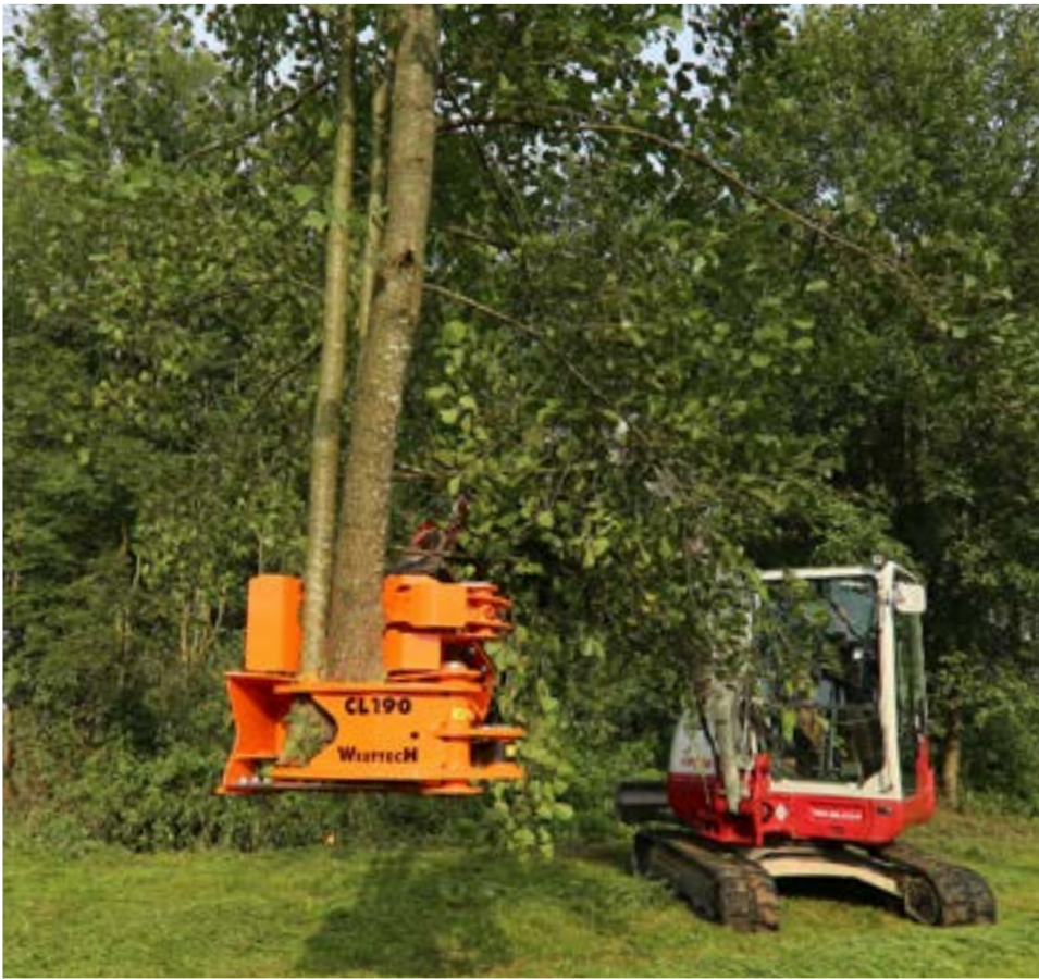
Woodcracker® CL is particularly suitable for the harvest of short rotation plantations.
